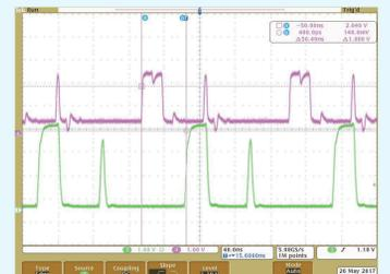
Round trip delay: 50 ns. Setup: 3U BNC - 3U VHDCI - 1m of VHDCI cable - 3U VHDCI - 3U BNC
