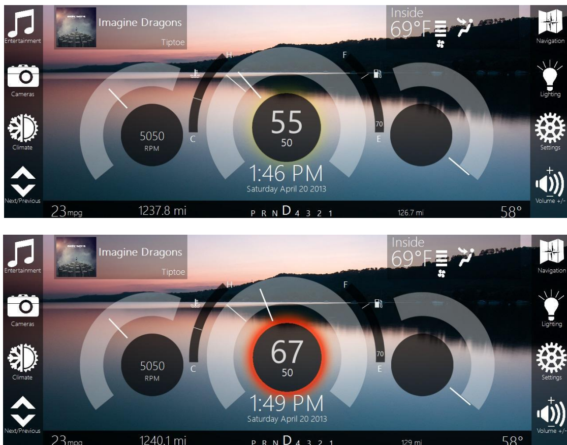
Figure 3: This figure shows how our enhanced speedometer works. When the driver is below the speed limit, there is no glow. Once they begin exceeding the limit, the glow begins to show, starting at yellow, becoming darker and darker, also indicating that the driving is breaking the speed limit.
